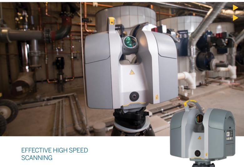
A powerful blend of speed, range and precision make the Trimble TX6 3D laser scanner the most productive scanner in its class. This entry level scanner delivers the high quality results you need for building MEP, BIM, engineering, construction and other applications.
