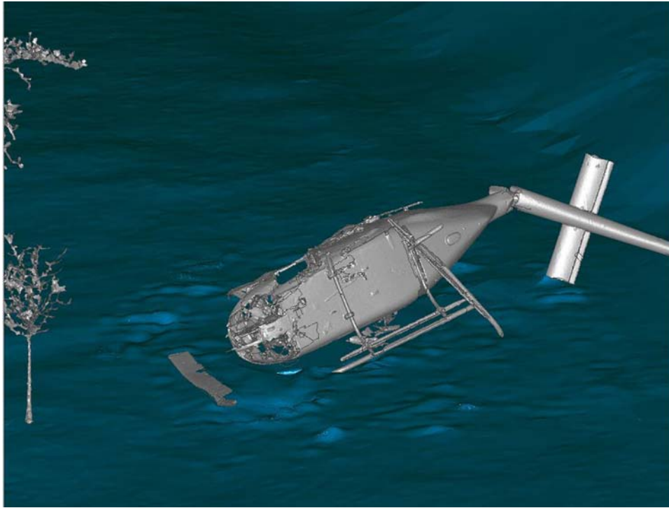
The accident scene modeled in Geomagic Studio from more than 50-million scan points.
