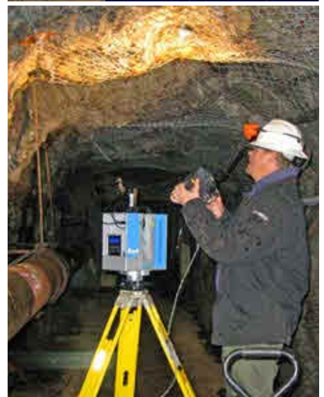
LASER SCANNING SERVICES WHEN YOU NEED THEM Maptek I-Site Services Manager, Scott Schiele manoeuvred the scanner and wagon in the confines of the Homestake drifts.
