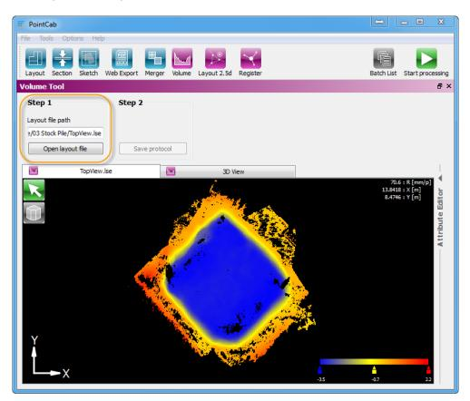
7. Activate the Volume tool and select the area for which the volume shall be calculated. The volume is immediately calculated and displayed.
