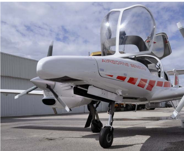
RIEGL NP680i: High-performance surveying technology fully included in the nose pod
