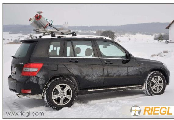
*RIEGL* VMX-250 mobile laser scanning system in action. The system can easily be mounted onto any commercial car roof carrier.
