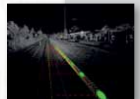
automated extraction of axis based analysis for detection of minimum distance to platform corner
