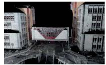
automatically cleaned-up point cloud
