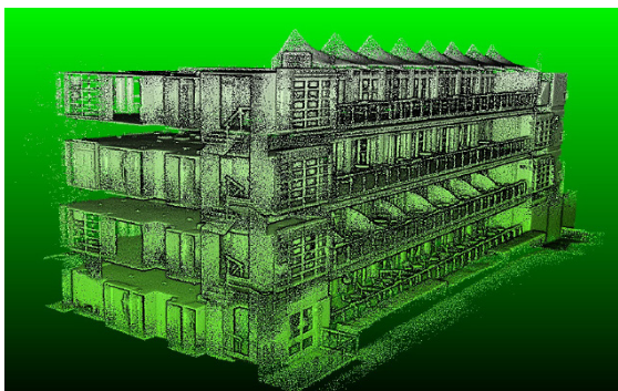
Scan of large pavilion building using handheld ZEB-REVO in just 30 minutes (data viewed in CloudCompare)
