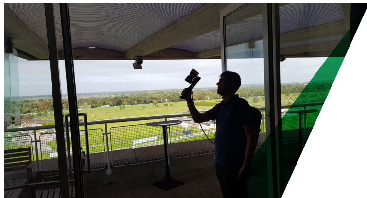
Capturing a large UK racecourse which has over 250 box rooms using the hand-held ZEB-REVO, project completed in under 3 weeks.
